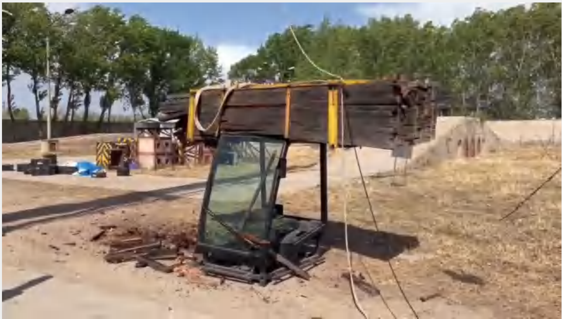
Over Head Guard full score passed impact test
