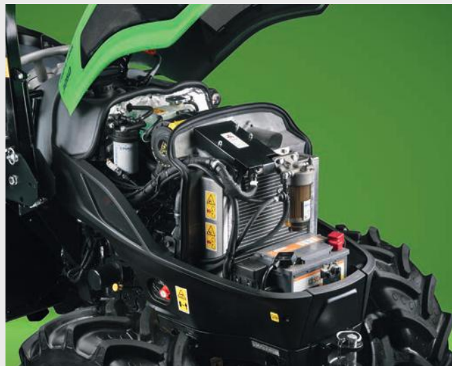
↑ Stage V compliant engines with Common Rail injection and power outputs up to 59 HP.
