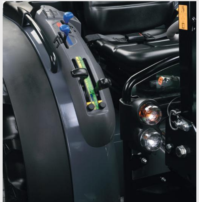
Rear lift with draft, position and mixed control.
