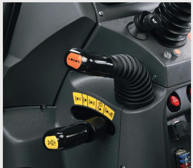
↑ Mechanical transmission with synchronized reverse shuttle.
