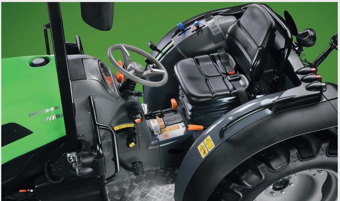
↑ ROPS version with platform suspended on Silent-Block mounts.
